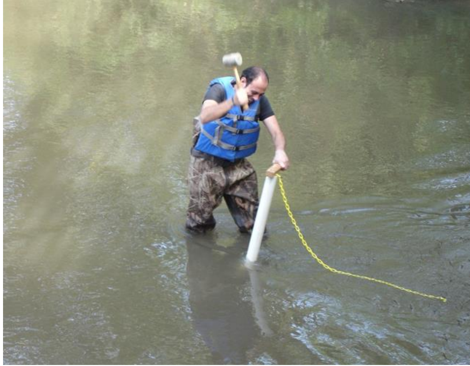
Figure 3-15. Stream bed material extraction process by hammering a PVC pipe into the bed. The material is removed by applying vacuum conditions using an expandable lid at the upper PVC tube end.
