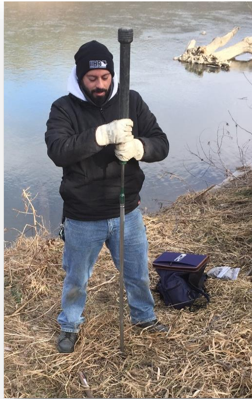
Figure 3-12. Soil sample extraction process from the floodplains using a hand auger with an attached sledge hammer.
