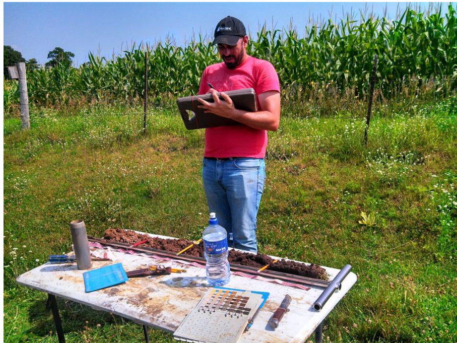
Figure 3-16. Each soil profile was divided into 0.20 m long segments and described before being placed into zip lock bags.
