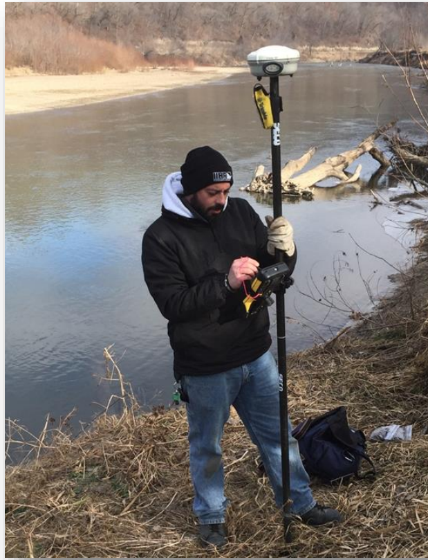
Figure 3-7. Field site survey along the identified CS using the Trimble GPS device.
